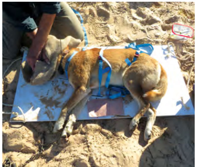
A Dingo being fitted with a GPS collar with a special accelerometer sensor that tracks and measures the velocity of its movements M Fischer
